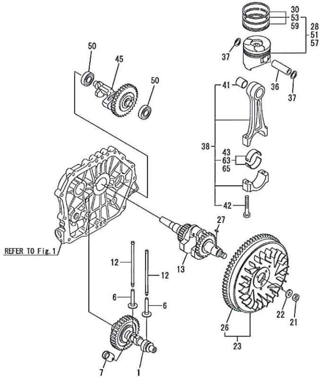
OCR10-G75900 4. CRANKSHAFT, PISTON & CAMSHAFT
